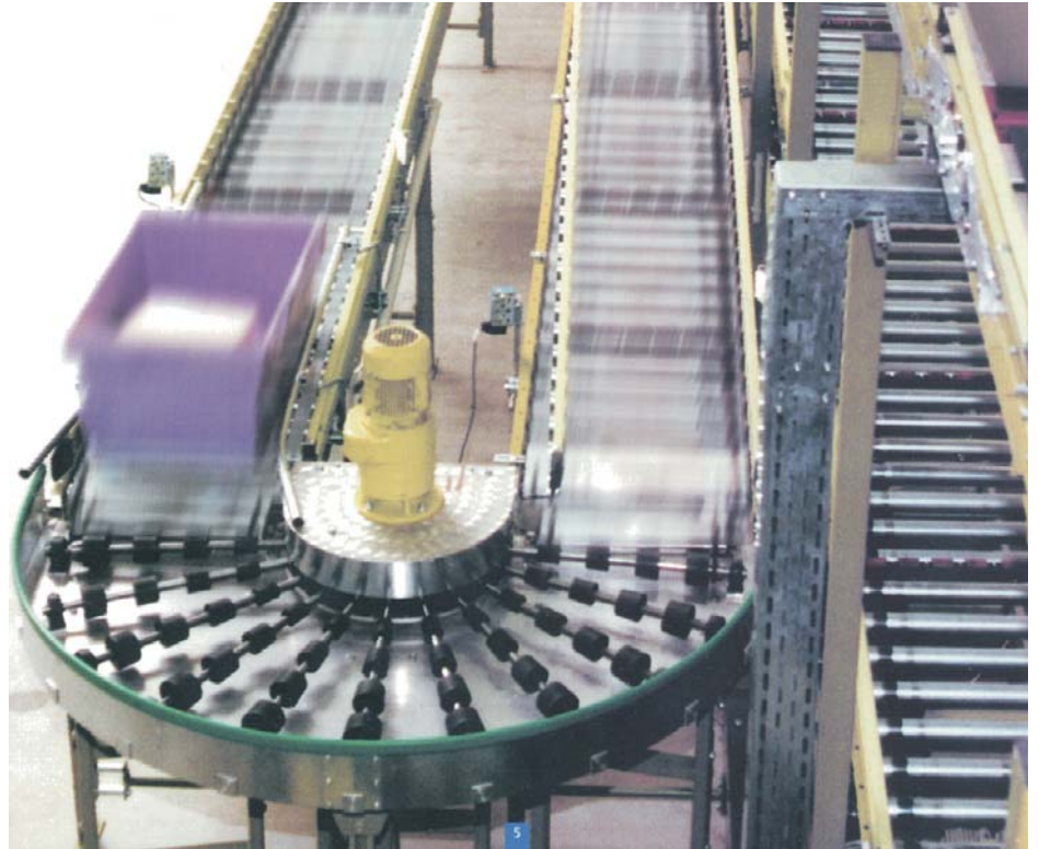
Roller conveyor with helical gear motor, brake with lockable hand ventilation and Harting connector
