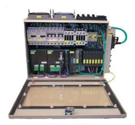
Die FLENDER TÜBINGEN-SIMATIC-EHB-control system is based on SIMATIC S7 standard components, by which the individual vehicle control systems communicate with the overriding central PLC via the internationally standardised PROFIBUS-DP. This takes over the vehicle tracking and soft control.
