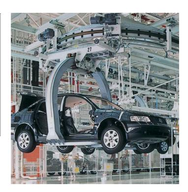
**Motox**<sup>®</sup>-N EHB gear motors offer an economical selection of sizes thanks to an optimum torque range of between 80Nm and 821Nm with finely graduated transmission ratios.
