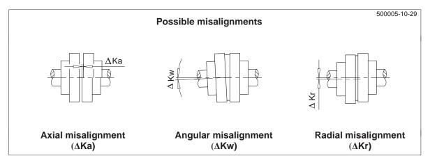
Alignment has to be done in two axial planes arranged perpendicular to each other. This can be done by means of a ruler (radial misalignment) and feeler gauge (angular misalignment). The aligning accuracy can be increased by using a dial gauge or, optically, by using a laser.
