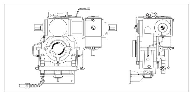
• The gear unit is mounted direct on the machine journal and secured against torsion with the torque reaction arm (the illustration shows a KHZP).
